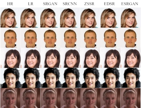
Fig. 7 Comparison of 2x reconstruction results of mainstream algorithms on MiniCelebA Test
